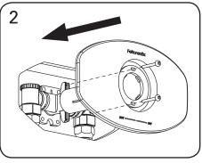
Position the wallplate over the valve outlet. Fit the two screws provided through each wallplate slot & into the valve body lugs. Tighten screws alternately - light pressure is sufficient to clamp the wallplate firmly to the wall.
