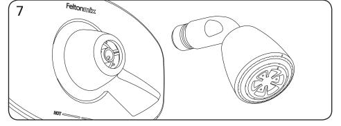
Screw showerhead into valve assembly - DO NOT OVERTIGHTEN. If necessary, unscrew showerhead part of a turn to bring it to the correct position. The o-ring seal fitted to the showerhead stem will ensure a watertight seal within 11/2 turns from fully tight. Do not use tape or hemp on the thread.
