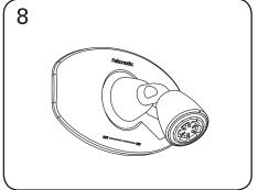
Check operation. Handle should swing from right to left from OFF to HOT. Total movement is about 130°.
