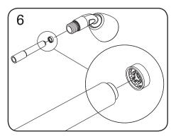
FOR EQUAL HIGH (MAINS) PRESSURE INSTALLATION, fit flow restrictor into showerhead with flow restrictor tool first.
