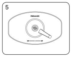
Handle should recess into the wallplate and match its contours. Ensure that the handle has about 10mm of engagement.
