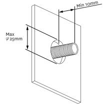
Install a  $\frac{1}{2}$ " male threaded connection at the recommended height on wall, ensuring that a minimum of 10mm of thread protrudes past the finished wall.
