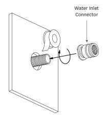
Apply thread tape (or similar) to the  $\frac{1}{2}$ " connection, then screw the top rail connector to the connection.
