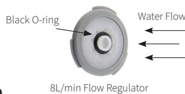
\*\*Ensure the flow regulator is fitted with the O-ring facing away from the hose (as shown), between Shower Elbow and Hose. This will comply with the WELS rating. Do NOT fit between handpiece and hose as this can overpressurise the hose and cause premature failure of the shower hose.
