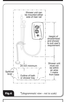
**IMPORTANT:** If installing onto a tiled wall, **ALWAYS** mount the unit on the surface of the tiles. **NEVER** tile up to the unit.
