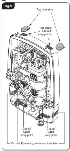
The backplate has removable top trims (top left and top right) that may be used for pipe entry and two additional sections (top left and top right) that may **ONLY** be used as a 'cut out' for top electrical cable entry (**fig.9**).
