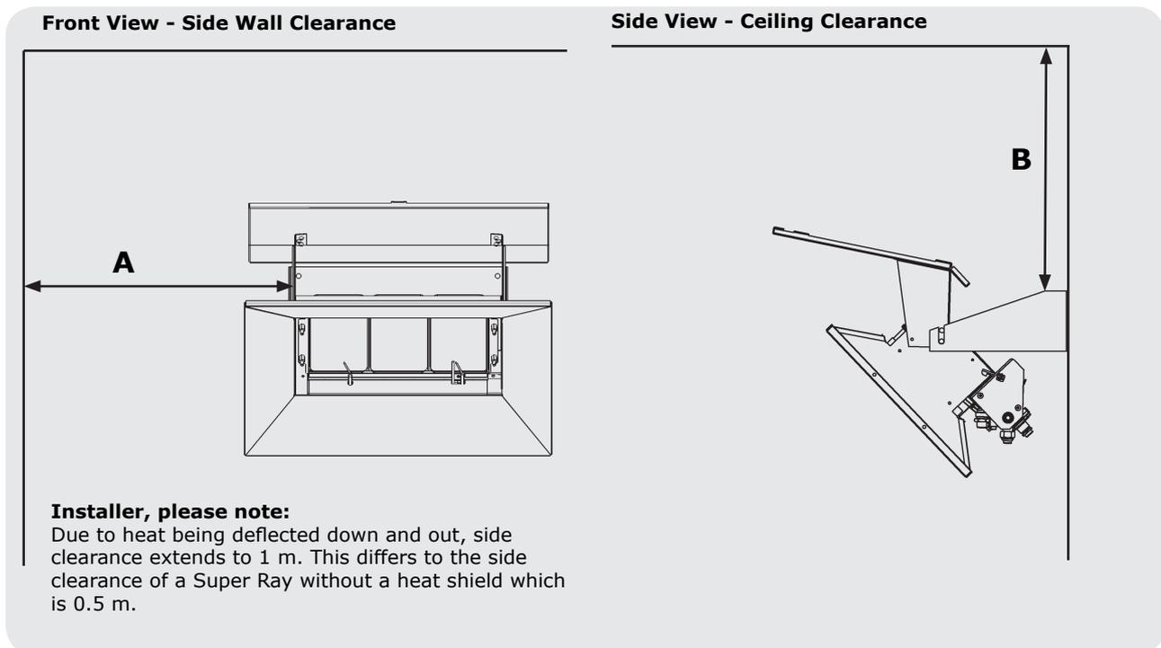
Angle of deflector is fixed and must not be altered. This is a safety feature.
