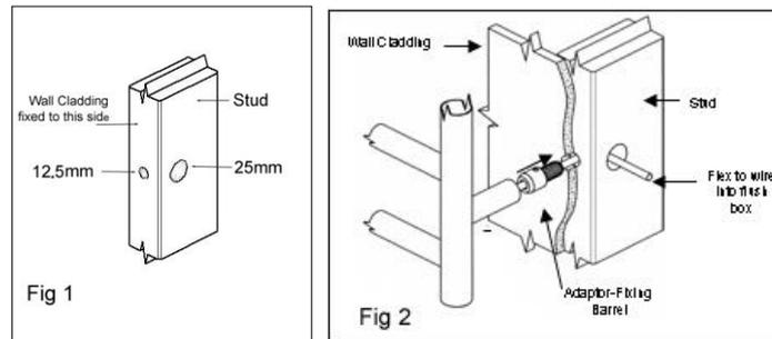
9. Place a pull through line from the flush box to the 12.5mm hole that can be picked up later once the wall cladding is in place
