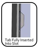
13. <u>DO NOT</u> perform the following instructions on Australian installations: To secure the front panel 4 to the pipe cover enclosure, open the four tabs at the top and bottom corners and secure with screws 7 and plastic washers 8. Next, close the tabs.
