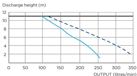
P1 - Output flow rate with one motor engaged
