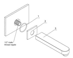
Insert the O Ring (1) into the base Place the base (2) over the water pipe nipple Apply plumber's sealant tape to the nipple Screw the spout (3) firmly to water piping and align correctly Remove the Aerator and turn on water and carefully check for leaks and let hot and cold water run for about one minute to clear possible debris.
