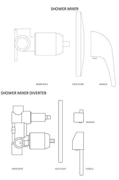
Mount the mixer body into the wall cavity securing it to the mounting stud. The distance between the rear mounting surface and the rear of the wall cladding and the cut out are as per the above
