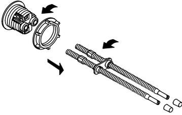
**2** *Using the push rod, measure the distance between the flush valve and the top of the tank lid. Mark this length and cut the push rod to length.*
