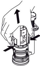
**2** Assemble flush valve by pressing it into the flush valve base so it snaps into place.
