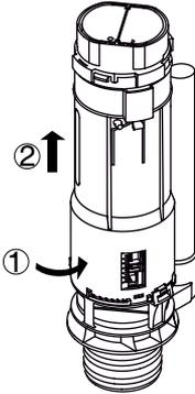
**2** Assemble flush valve by pushing straight down into the canister and turning left.
