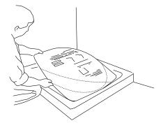
Mark and drill holes required for outlet fittings as per *figure 7*.
