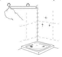
Position wall in place. Check fit to ensure wall fits squarely into corner as per *figure 8.* Tape edges to hold into position.
