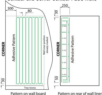
Fig.13: Adhesive pattern for Side Recessed Walls
