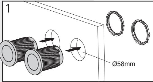
Mark out and drill holes for the Custom Buttons in the desired position. Round buttons require a hole diameter of 58mm and are suitable for panels up to 55mm thick.
