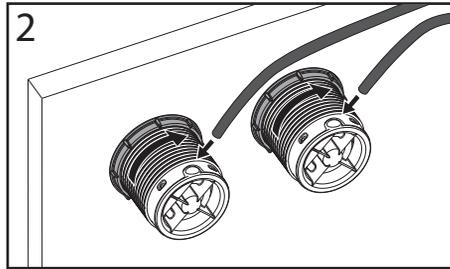
Insert the Button Assembly and tighten Mounting Nut up from behind. Push the hoses into the Button Assemblies ensuring the hoses from the cistern are correctly matched with the half flush and full flush buttons
