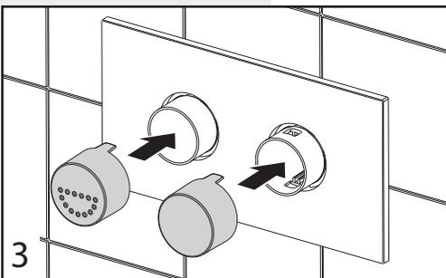
Once the Face Plate has been locked, the Button Caps can be clipped on. Ensure the half flush button cap is on the left.
