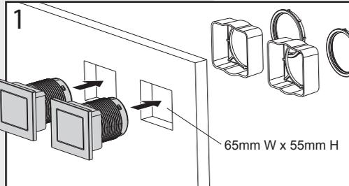
Mark out and drill holes for the Custom Buttons in the desired position. Rectangle buttons require a hole size of 65mm W x 55mm H and are suitable for panels up to 55mm thick.
