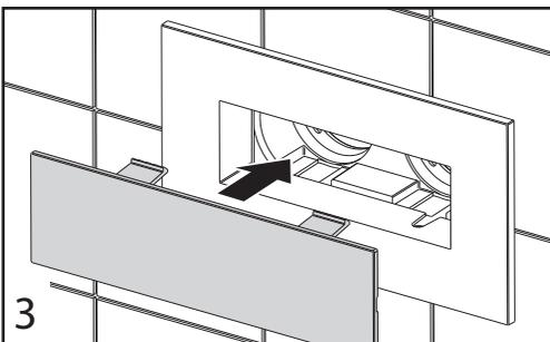
Once the Face Plate has been locked, the Blanking Panel is simply clipped into place.
