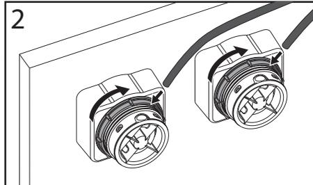
Insert the Button Assembly and tighten Mounting Nut up from behind. Installations where the thickness of the mounting plate is less than 26 mm will require the additional Spacer. Push the hoses into the Button Assemblies ensuring the hoses from the cistern are correctly matched with the half flush and full flush buttons
