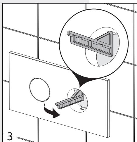
Depress the full flush button and using the supplied Allen Key, lock the Face Plate to the Mounting Panel - there are two locks - top.....
