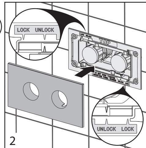
Ensure the Locking Racks are in the 'UNLOCK' position, then assemble the Face Plate to the Mounting Panel
