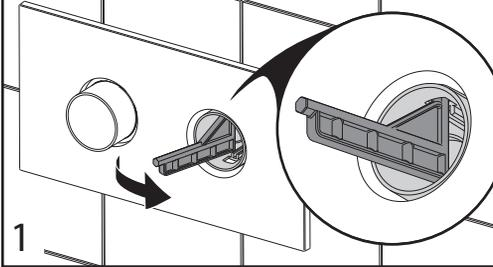
The installation method is identical to the Round Button Panel Assembly except that it will be provided without the button caps attached. To lock the Face Plate, depress the full flush button so the Allen Key can be used through the slot in the button slider - top.....
