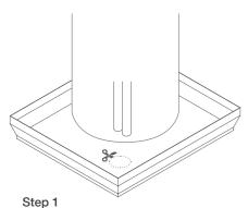
Using a hole saw cut a outlet in the desired location on the safe tray.
