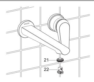
Ensure that all coupling nuts are tight. Ensure that the lever handle is in the off position.
