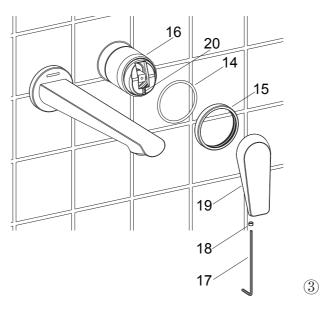
Slide the escutcheon(15) with O-ring(14) onto the valve base(16).
