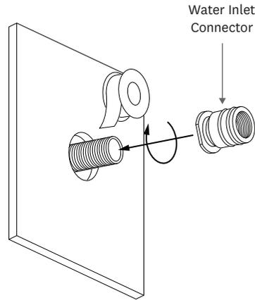
Apply thread tape (or similar) to the 1/2" connection, then screw the top rail connector to the connection.
