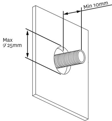
Install a 1/2" male threaded connection at the recommended height on wall, ensuring that a minimum of 10mm of thread protrudes past the finished wall.
