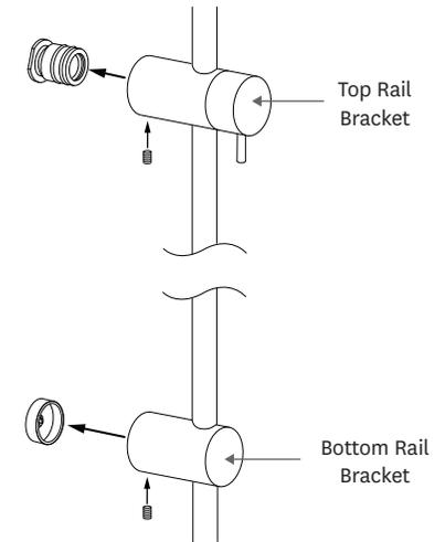
Check the grub screws are wound out. Push the rail brackets onto the top and bottom rail connectors until they are against wall. Secure with grub screws.
