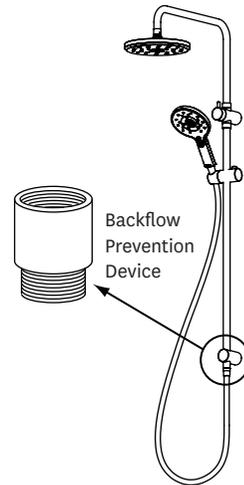
Make sure a washer is in both ends of the hose. Screw hose onto lower outlet on wet rail, attach handset and place firmly in holder. Tilt and rotate head to the desired position.
