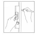
Pre drill three equally spaced clearance holes (i.e. top, bottom and centre) in the Wall Receivers using a 4.5mm drill bit. Reposition the Wall Receivers onto the wall. Drill into the wall through the clearance holes using a 3.0mm drill bit. **N.B.** The holes preferably locate into a stud or nog. As an alternative, a toggler system can also be used.
