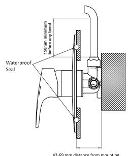
42-69 mm distance from mounting stud to outside face of wall lining
