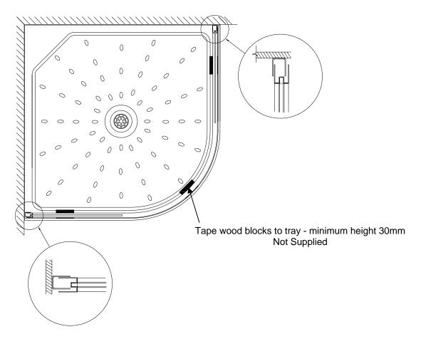
Lift Door Frame assembly onto the wood blocks and place into Wall Receivers as shown When lifting the Door Frame assembly, hold it by the vertical edges of the glass or door frame. **Under no circumstance lift by the Head and Sill as this may cause the glass to fall out of the glazing gaskets**
