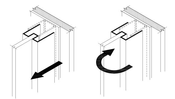
While still resting on the wood blocks "Spring" the Door Frame assembly so it sits over the legs of the Wall Receiver. Repeat for other side.
