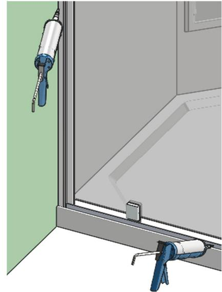
**17)** For White Showers only - take the Cleaning Towelette and wipe the surfaces of the Powder coated profiles where Silicone will be applied Allow to dry (1-2 minutes)
