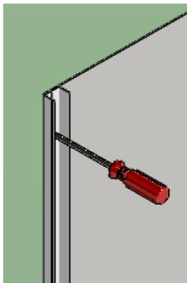
4) Secure the Wall Receiver to the wall using the No.6 x 38mm stainless steel screws
