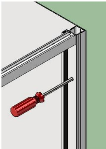
**9)** Secure the Wall Receiver to the wall using the No.6x 38mm stainless steel screws.
