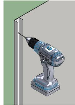
1) Determine which side the Door is to be hung. Position one of the Door Wall Receivers hard against the inside edge of the tray up-stand.
