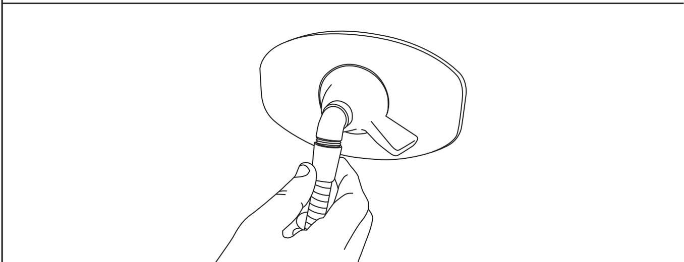
3. **For Mains Pressure, fit flow restrictor into the handpiece first.**
