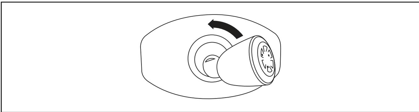
1. Remove the shower head from the existing Feltonmix wallset by gripping the shower head stem and turning it anti-clockwise.
