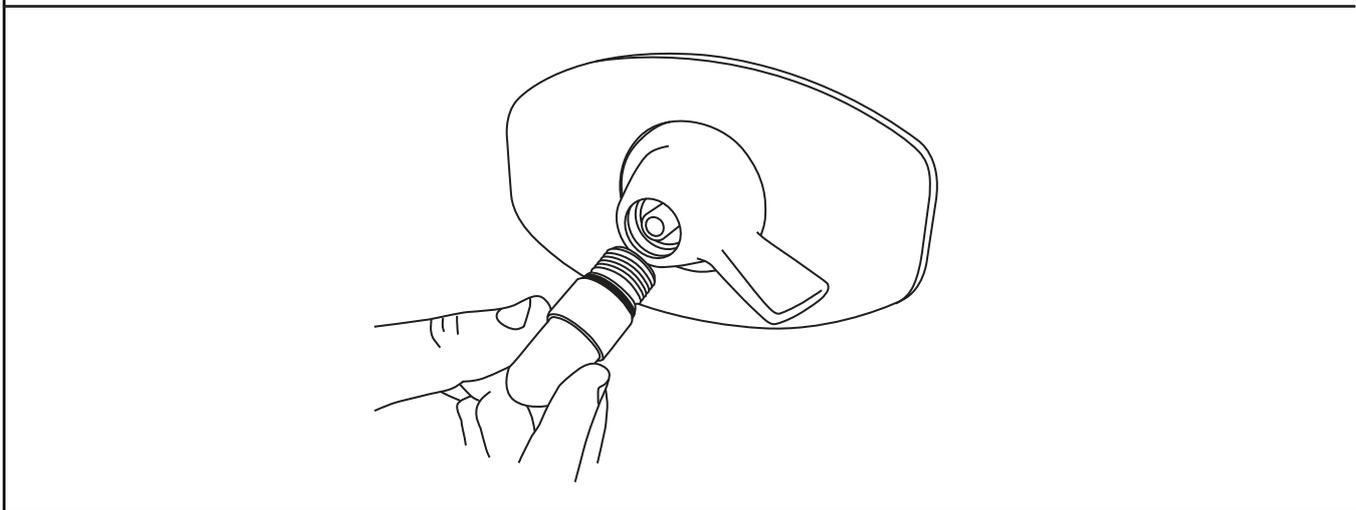
2. Screw the elbow end with the black 'o-ring' into the wallset. The plastic flange provided will not be needed for this conversion.
