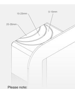
Breakaway elements above to suit varying wall finish thickness'. 35-40mm doesn't require any breakaway sections to be removed.
