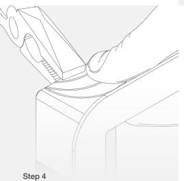
Breakaway required section of faceplate to suite finished wall thickness. Support required sections with thumb and forefinger, use a set of pliers to breakaway undesired element(s). Tidy area with deburring tool.
