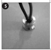
Take the threaded mushroom and screw down onto the exposed threaded rod. Pull the wire through and attach to the wire connection on the individual bar.
