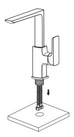
3 Slide on the rubber and steel washer, then the fixing nut, and while holding the mixer in place tighten using a wrench.
