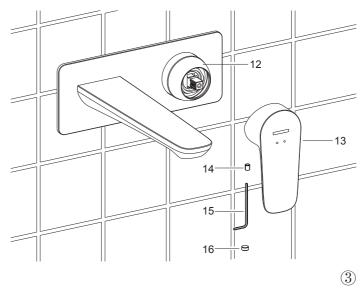
Turn off the valve, and loosen the screw(14) in the handle(13) with 2.5mm hex wrench(15). Install the handle onto the valve base(12) with it downwards. Tighten the screw with hex wrench and press the plug button(16) to the hole.
