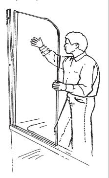
Check that the bottom of the glass is parallel with the top edge of the bath.
