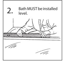
Position wall retainer flush to the outside of the bath and vertical using a spirit level.
