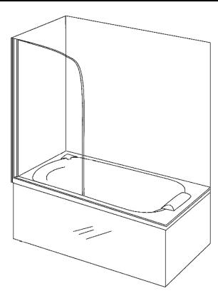
Bath screens must be installed in situations where the floor of the bathroom has a waterproof membrane installed. For New Zealand, the bath screen must be installed in accordance with NZBC E3/AS1 clause 3.1.1. For other countries, the bath screen must be installed in accordance with local building codes.
