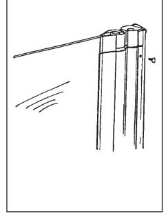
6. Select the correct seal extension and slide into place as shown.
