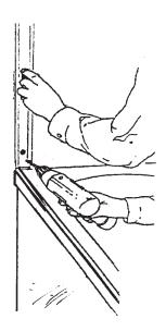
Mark the position of the three holes in the wall retainer and, using a 3mm drill bit, drill the holes for the No.  $6 \times 1^{1/4}$ " screws.
