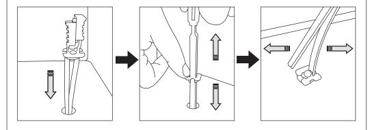
2 Insert the mounting plate into the mounting holes.
