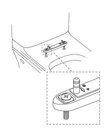
3 Position the mounting plate and tighten the screws.
