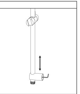
1. Untighten the grub screws from the top and bottom of the rail with a 2.5mm allen key and remove the brackets.
