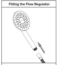
1. Supply as is with the Flow Regulator prefitted and screw on the hose.
