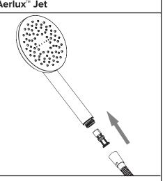
Select the Purple or Orange Aerlux™ Jet and fit into the handpiece before screwing it onto the hose.
