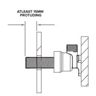
2. Cut and fit 1/2" BSP with atleast 15mm protuding from the finished wall. Use seal tape when threading into wingback.
