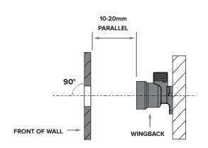
Ensure the wingback when fitted is parallel and square to the finished wall lining as shown
