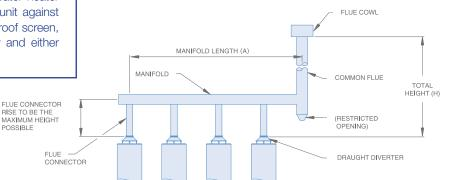
Multiple Manifold Flue System
