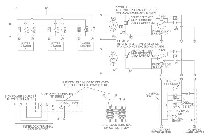
Intermittent PowerFlue Fan Control - Multiple Water Heater Rheem 624 Series & Raypak Type B Series.
