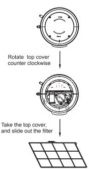
When installing the top cover please refer to the direction of arrow, after assembling it should be line up.
