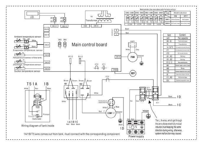
T3: Evaporator Temp. Sensor T4: Ambient Temp. Sensor
