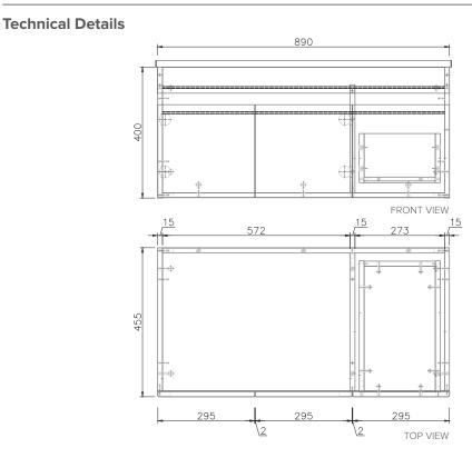
Note: All measurements shown are in millimetres. Sizes are nominal.
