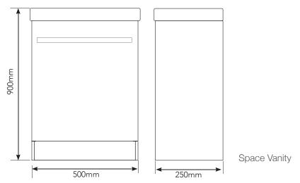
NB: Drawings indicate the technical measurements only and is not a reflection of how the unit will look.
