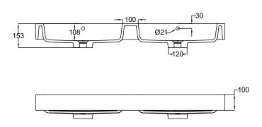
NB: Drawings indicate the technical measurements only and is not a reflection of how the unit will look.
