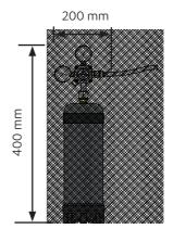
Secure cylinder vertically to a robust surface with the hook & loop strap and bracket supplied
