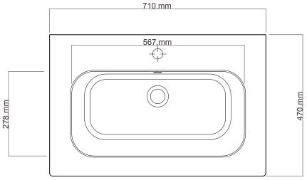
NOTE: Drawing indicate the technical measurement only and is not a reflection of how the unit will look.
