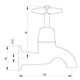
CONSTRUCTION: Brass body CLASSIFICATION: Suitable for all pressure systems INLET CONNECTIONS: 1/2 " BSP Female WORKING PRESSURE: 10 - 500kPa DIMENSIONS FOR FITTING: see installation manual OPERATING TEMPERATURE: 5 °C - 80 °C
