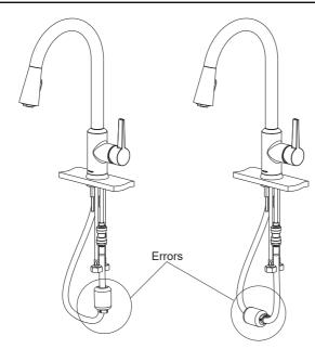
Put the weight(12) and clip(13) onto the pull hose(7). Connect the pull hose and the connecter(10). Adjust and position the weight and clip. **Note:** Don't over distort the hoses. Please avoid the wrong installation for the weight and clip as shown in the above.
